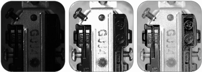
Registration (HDR): Short exposure, long exposure, result
