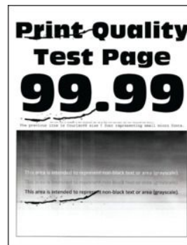
Repeating defects on page 213
