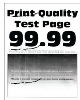
Repeating defects on page 205
