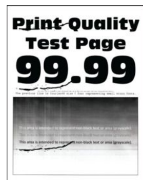
Repeating defects on page 141
